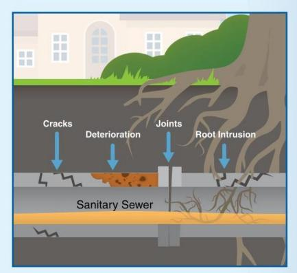
**Infiltration** is clear water that gradually enters the wastewater system below ground through cracks and openings in sewer service lines and joints, and public sewer mains and deteriorated maintenance holes.
