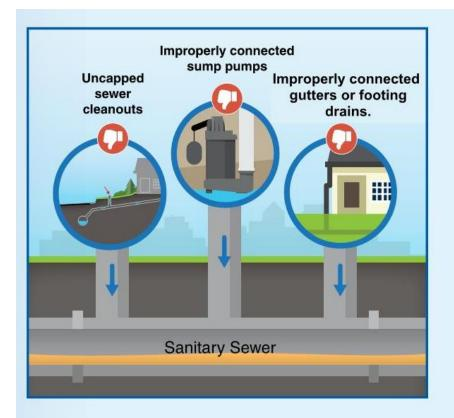
**Inflow** is clear water that quickly enters the wastewater system after rainfall events from sources such as sewer cleanouts, sump pumps, gutters, building foundation drains, and broken maintenance hole covers.
